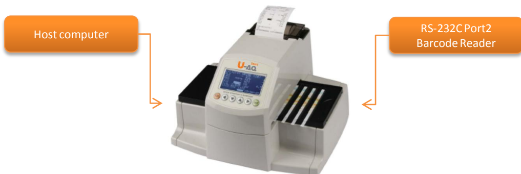
*Connection diagram between U-AQ Smart and Host Computer*
